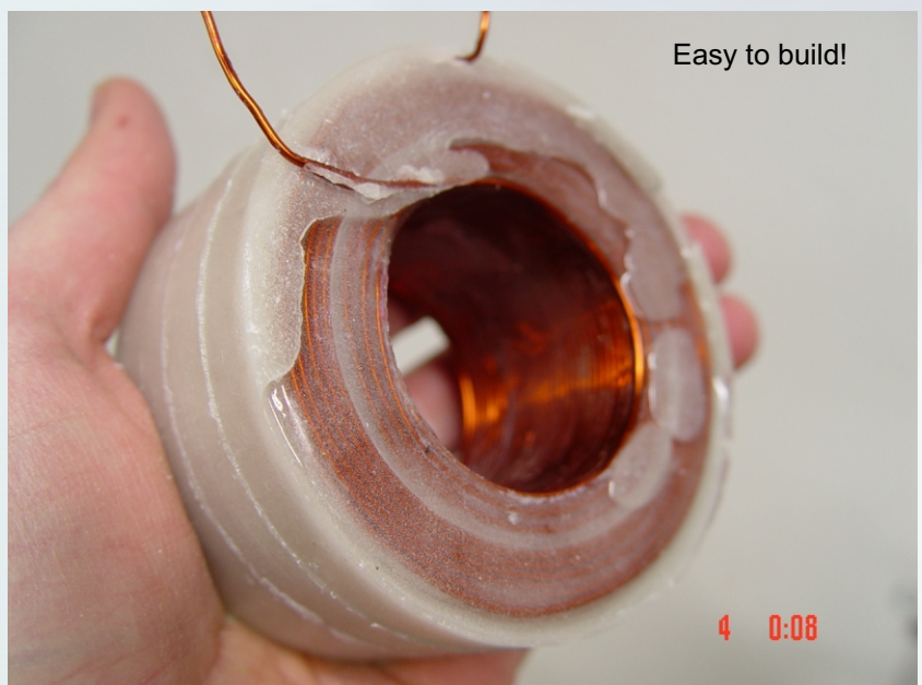
A close up of one of our special Sp500 coils with a two part epoxy coating. From our Sp500 Model # 4 included in the plans.
